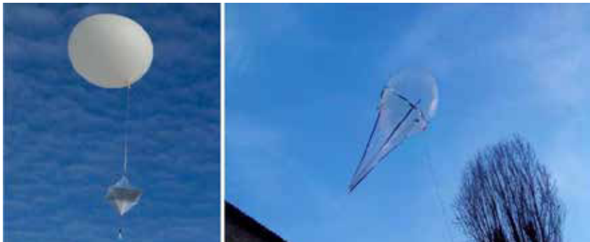
Figure A.2.31 – Balloon with a corner reflector (false target); tethered observation balloon
