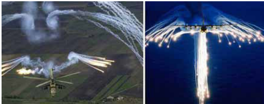
Figure A.2.63 – Heat traps released from helicopter and from aircraft
