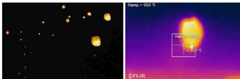
Figure A.2.20 – A group of sky lanterns; view of a sky lantern in a thermal imager
