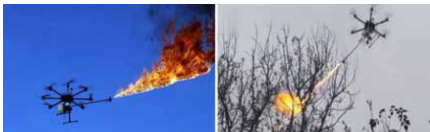
Figure A.2.54 – UAV flamethrower in operation
