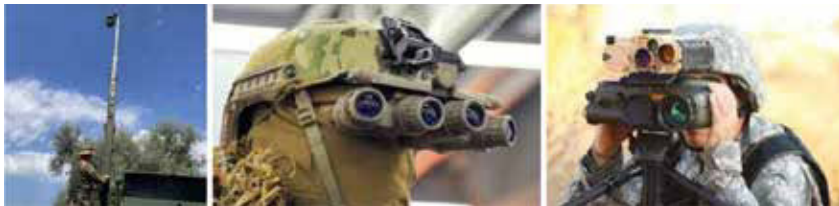
Figure 1.2 – Examples: A stationary video camera; an individual night vision device; a portable handheld visual reconnaissance system
