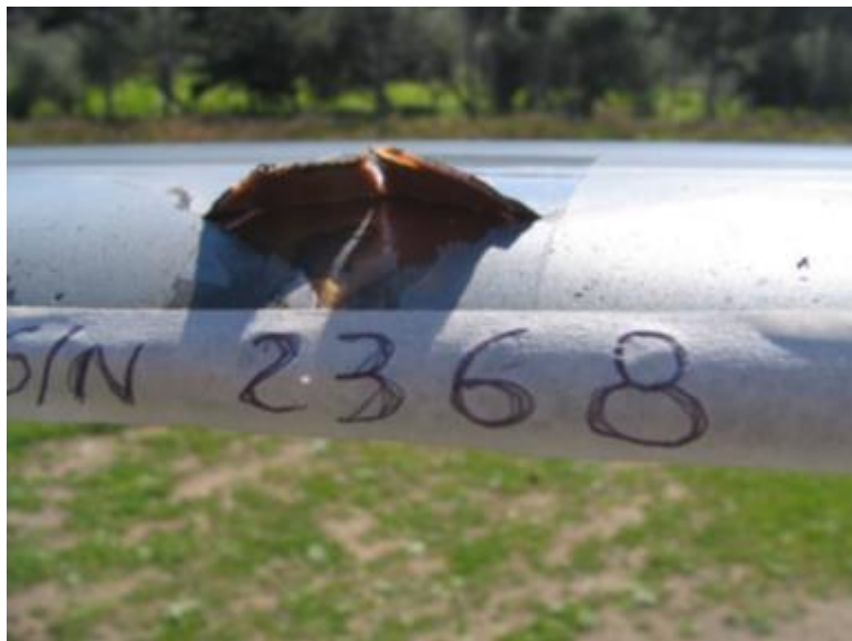
Figure 7: Photo of damaged helicopter blade (source: Francesco Venerando).
