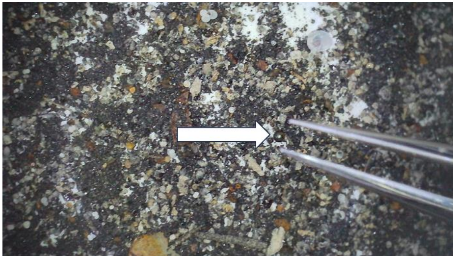
Рис.17. Collected material from the magnetic sled at IM1's site, showing a 0.4-millimeter diameter iron-rich spherule (white arrow) amongst a background of shell hash and other debris. The collection of spherules by the expedition had a yield per background mass that increased significantly the count of spherules near IM1's path. The heatmaps below show that the spherules collection had three high-yield regions, colored in yellow, relative to the control regions colored in purple, potentially reflecting the three flares from IM1's light curve .
