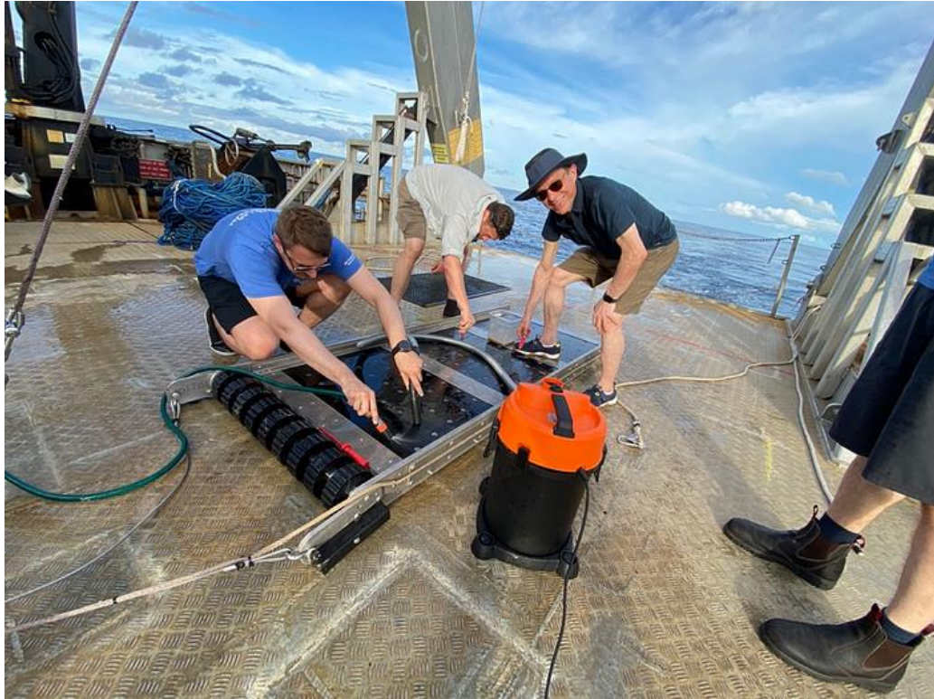
Рис.16. Vacuum cleaning and scraping of the sled's magnets by team members J.J. Siler (left) and Avi Loeb (right).
