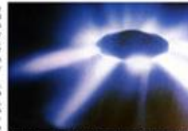
Figure 29. Picture of RF discharges. The shiny edge of this disk-shaped model made of an electrically conducting material makes radial RF discharges looking like "truncated light rays".
